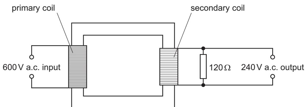
What is the power dissipated in the resistor and what is the current in the primary coil?
