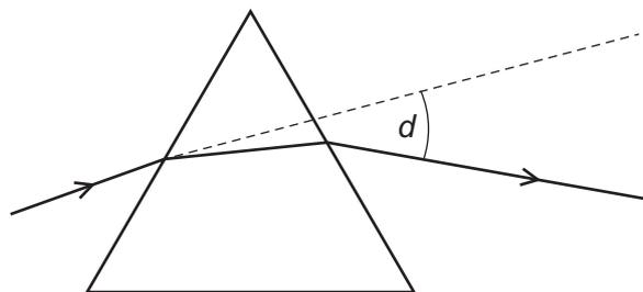
The deviation angle  $d$  is measured for light rays of different frequency, including blue light and red light.
