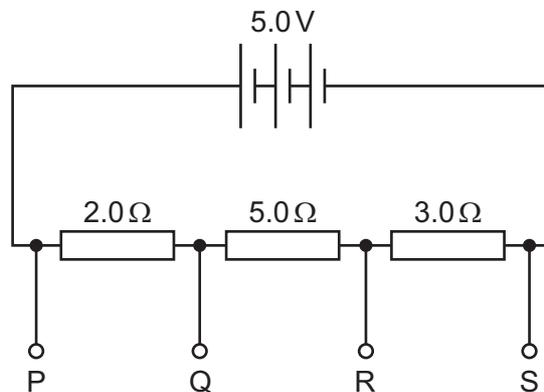
Between which pair of terminals is there a potential difference of 1.5V?
