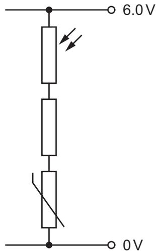
Under which conditions is the voltage across the fixed resistor the greatest?
