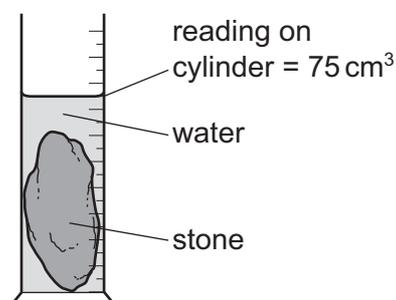
The volume of water in the cylinder before adding the stone is 15 cm<sup>3</sup> and the stone has a mass of 90 g.
