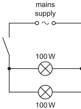
How much electrical energy is supplied by the mains when the switch is closed for 36 minutes?
