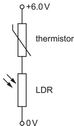
The thermistor has a resistance of  $6000\ \Omega$  in a cold room and  $1000\ \Omega$  in a warm room. The LDR has a resistance of  $2000\ \Omega$  in dim light and  $500\ \Omega$  in bright light.
