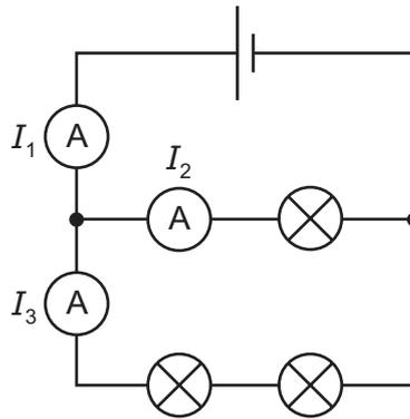
The readings on the ammeters are  $I_1$ ,  $I_2$  and  $I_3$ .
