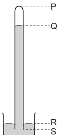
The mercury level in the tube falls, leaving a vacuum at the top.
