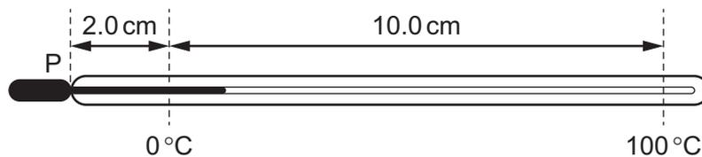
Measuring from P, how long is the liquid column at 30°C?
