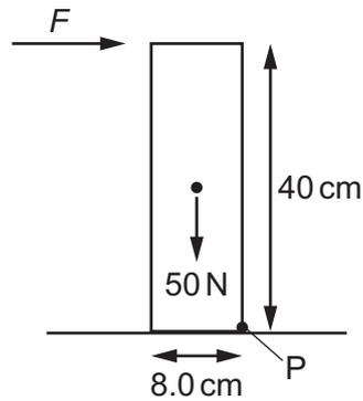
Which horizontal force  $F$  just makes the block start to rotate about P?
