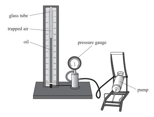
Air is trapped in a glass tube of uniform cross-sectional area. A pump forces oil into the base of the glass tube. This forces the air into a smaller volume. The pressure of the trapped air is displayed on the pressure gauge.
