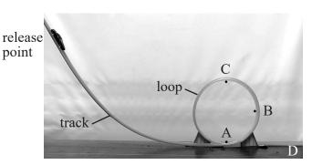
If the release point of the car is high enough, the car moves fast enough to pass point C and complete the loop, continuing to the end of the track at point D.
