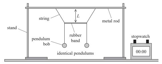
One pendulum is set in motion. The amplitude of oscillation of this pendulum decreases to zero as the rubber band transfers energy to the other pendulum, which oscillates with increasing amplitude.
