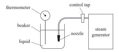
The control tap adjusts the rate of flow of steam from the nozzle. The steam heats the liquid in the beaker.
