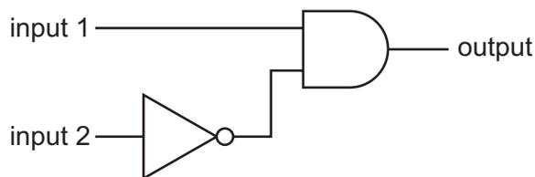
Which truth table represents the operation of this combination of logic gates?
