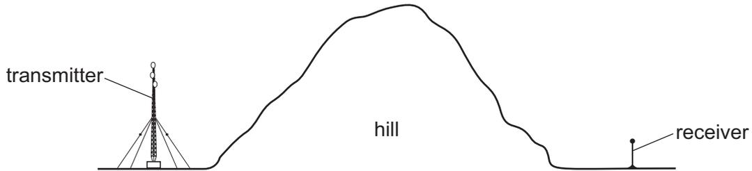
The receiver picks up the signal from the transmitter even though the radio waves do not travel through the hill.
