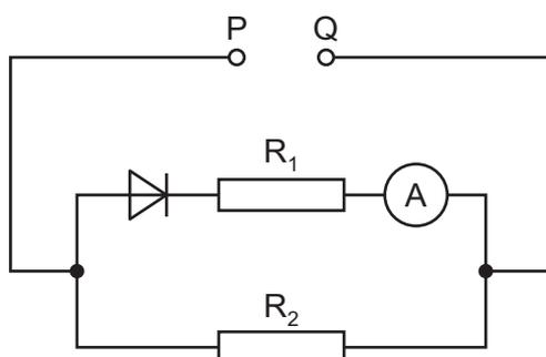
Under which circumstances does the ammeter show a reading other than zero?
