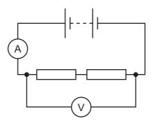
The voltmeter reading is 2.2 V and the ammeter reading is 0.25 A.
