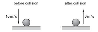
The collision between the ball and the floor lasts for 0.50 s.
