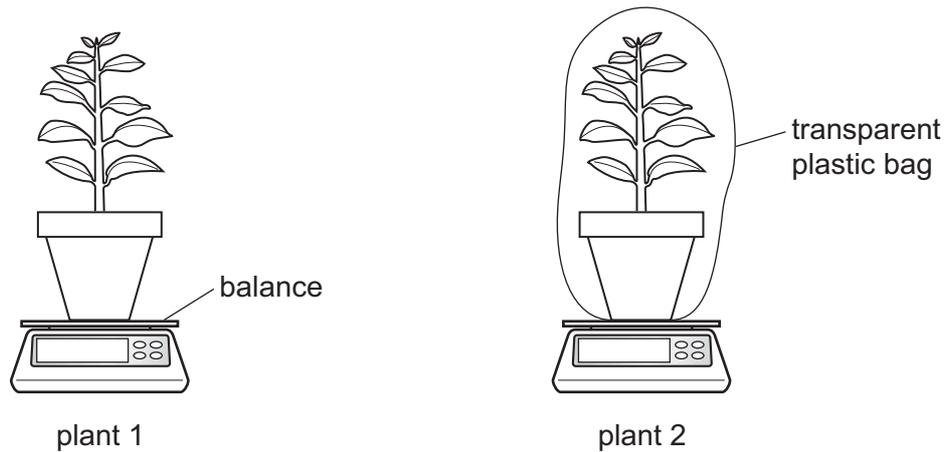
Plant 1 is not covered. Plant 2 and its pot are covered by a transparent plastic bag.
