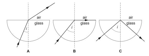
(a) (i) State in which diagram, **A**, **B** or **C**, the angle of incidence is equal to the critical angle.
