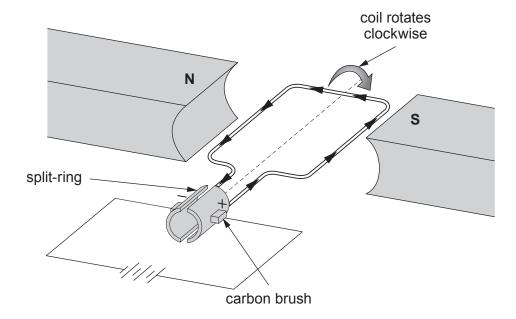
The direction of the force on the coil is given by using Fleming's left-hand rule.
