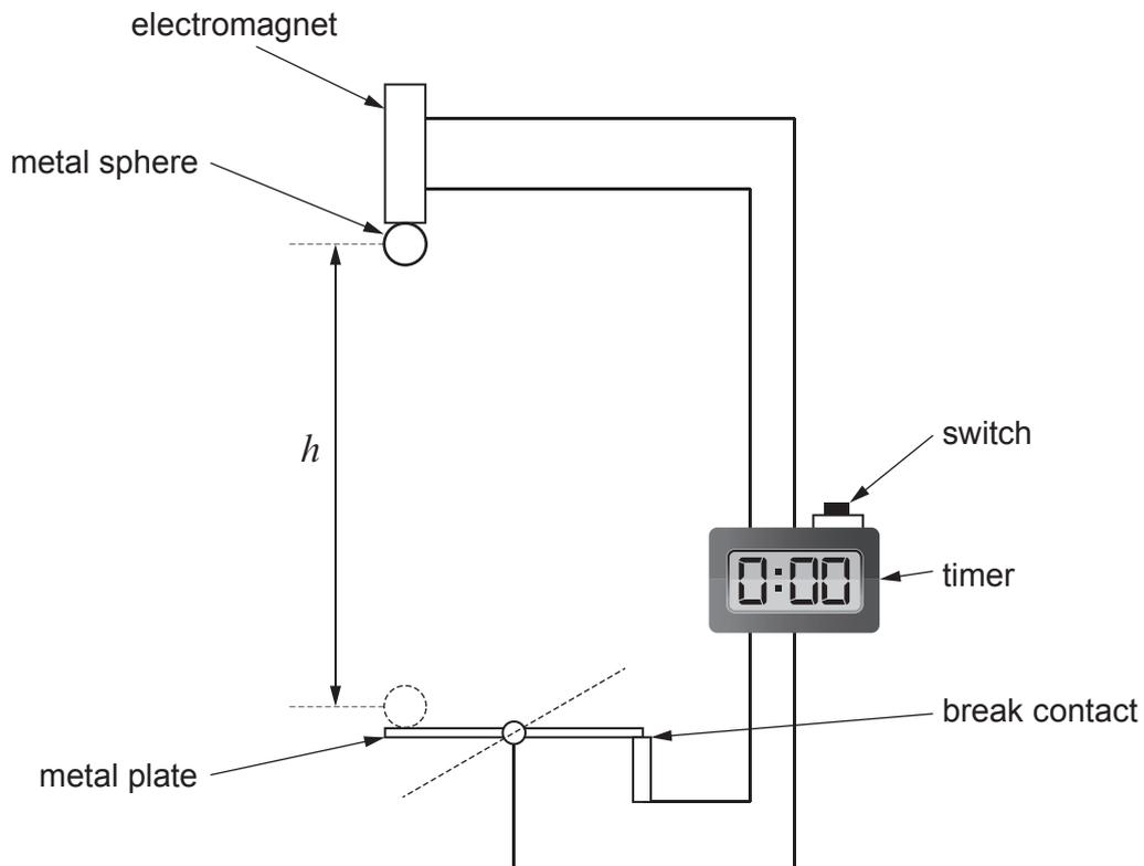
When the switch is pressed, it starts the timer and disconnects the electromagnet, almost instantly releasing the metal sphere. When the sphere hits the metal plate it breaks the circuit, stopping the timer. The time taken for the metal sphere to fall through a range of different heights,  $h$  is measured.
