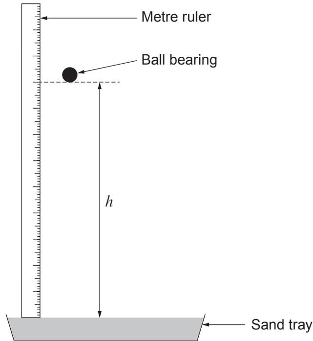
Richard dropped the ball bearing and measured the diameter,  $d$ , of the crater it left in the sand. He repeated this for a series of different heights,  $h$ . To ensure his results were repeatable he carried out the experiment three times from each height and obtained the following results.
