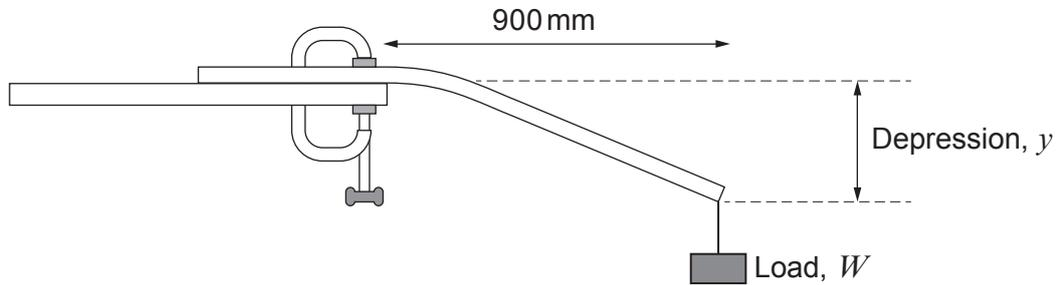
The depression of the cantilever was measured on loading and then unloading using a metre ruler of resolution  $\pm 0.1$  cm. The results were recorded in the table below.
