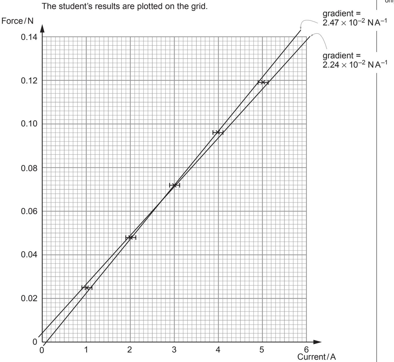
(ii) Calculate the mean value of the gradients ( $2.47 \times 10^{-2} \text{ NA}^{-1}$  and  $2.24 \times 10^{-2} \text{ NA}^{-1}$ ) and its **percentage** uncertainty. [3]
