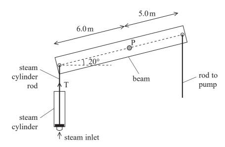
(a) The beam has a constant thickness and a mass of  $3.05 \times 10^4$  kg. The length of the beam is 11.0 m. The pivot P is positioned 6.0 m from the steam cylinder end of the beam.
