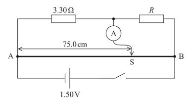
A metal slider S can be moved along the nichrome wire and pressed firmly against it to make an electrical connection.
