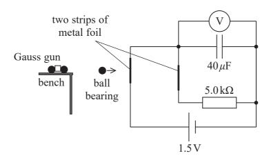
As the ball bearing left the gun, it broke the first foil strip at its centre so that the capacitor started to discharge. When the ball bearing broke the second foil strip the capacitor discharge stopped.
