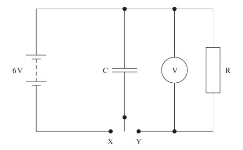
The student used the switch to connect C to X to charge the capacitor. She then connected C to Y to discharge the capacitor through R.
