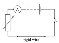
With the switch open, the balance was set to zero. When the switch was closed a current I in the circuit was recorded by the ammeter and the reading on the balance increased.
