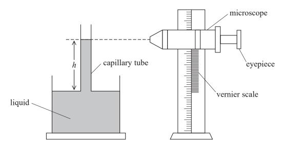
(a) The student used a capillary tube with an internal radius r equal to  $0.10 \, \text{mm}$  and recorded the following readings from the vernier scale.
