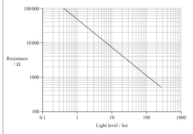
The transistor switches on when the potential difference across the input increases above 0.7 V. This should happen as the light level reaching the LDR increases above 30 lux.
