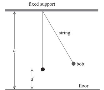
As the student was unable to measure the length of the pendulum directly, she measured the distance d from the bob to the floor.
