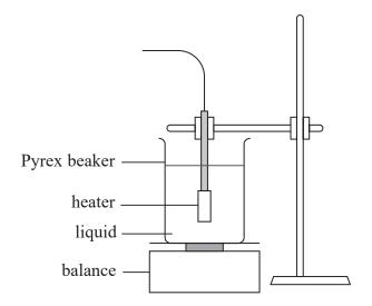
(a) She connected the heater into a circuit and took measurements of the potential difference V and the current I for the heater.
