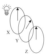
Filter Z is then rotated clockwise and the intensity of light emerging from Z is measured.
