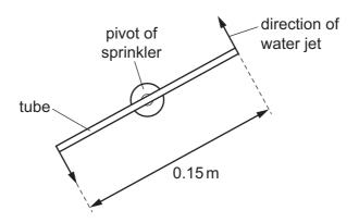
The sprinkler consists of a tube of length 0.15 m. The tube is pivoted in the middle and spins in a horizontal plane as it lets out jets of water from each end. The two water jets are in opposite directions to each other. Each water jet exerts a horizontal force of 3.0 N on the tube at right angles to the tube.
