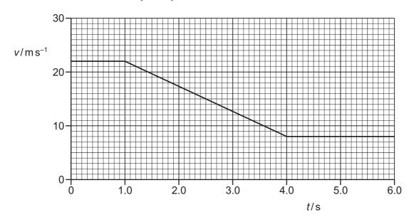
The brakes of the car are applied from  $t = 1.0 \,\mathrm{s}$  to  $t = 4.0 \,\mathrm{s}$ .
