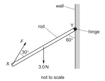
A force F acts at an angle of  $30^{\circ}$  to the rod at end X. The rod has a weight of  $3.0\,\mathrm{N}$  and is in equilibrium.
