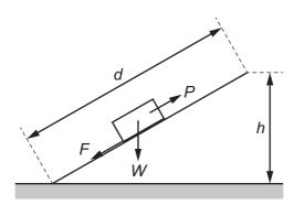
The purpose of the slope is to raise the box vertically.
