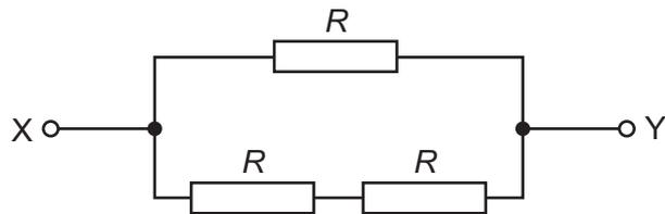
The total resistance between points X and Y is  $8.0\ \Omega$ .
