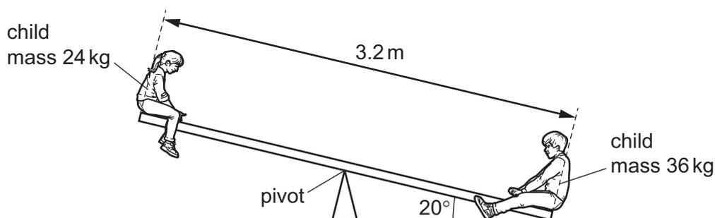
One child has a mass of  $24\text{ kg}$ . The other child has a mass of  $36\text{ kg}$ . The heavier child causes one end of the beam to permanently rest on the ground, so that the beam makes an angle of  $20^\circ$  to the horizontal ground.
