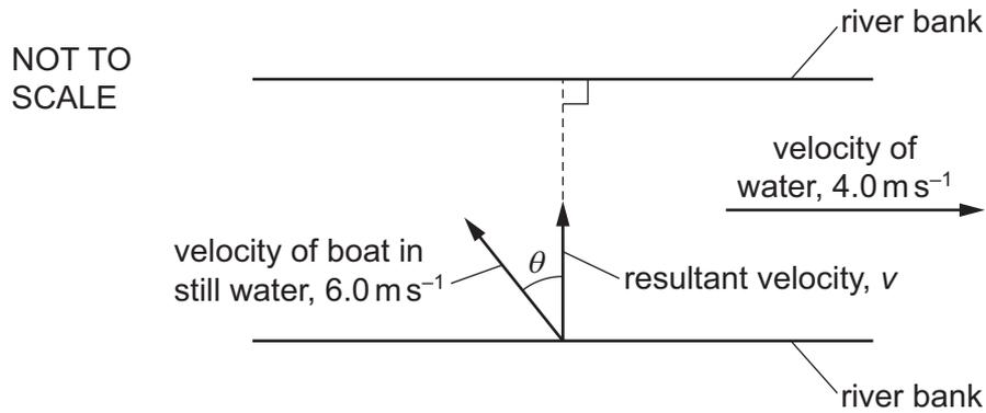
In still water, the speed of the boat is  $6.0 \text{ m s}^{-1}$ . The boat is directed at an angle  $\theta$  to a line perpendicular to the river banks. The resultant velocity  $v$  of the boat is in a direction perpendicular to the river banks.
