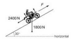
As the motorbike is travelling at constant speed up the slope:
