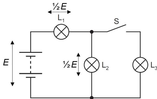
With the switch S closed, the parallel combination of lamps  $L_2$  and  $L_3$  now have a combined resistance of half the resistance of one of the lamps. The p.d. across lamp  $L_1$  is now twice as much as the p.d. across  $L_2$  and  $L_3$ . It has increased from  $\frac{1}{2} E$  to  $\frac{2}{3} E$ , so lamp  $L_1$  will be brighter. The p.d. across lamp  $L_2$  has decreased from  $\frac{1}{2} E$  to  $\frac{1}{3} E$  so lamp  $L_2$  will be dimmer.
