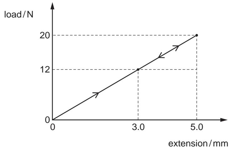
How much strain energy is released during the unloading process?
