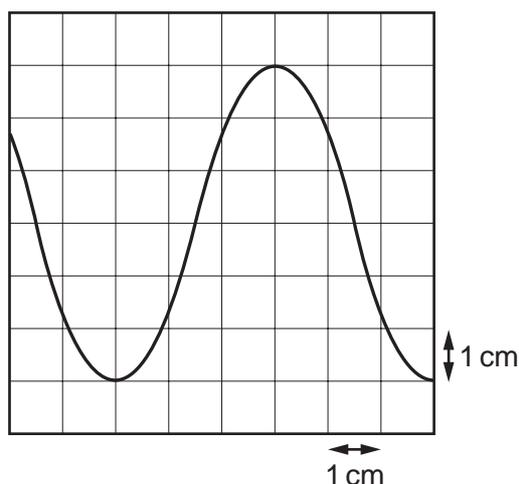
The time-base setting is  $0.5 \text{ ms cm}^{-1}$  and the Y-plate sensitivity is  $0.2 \text{ mV cm}^{-1}$ .
