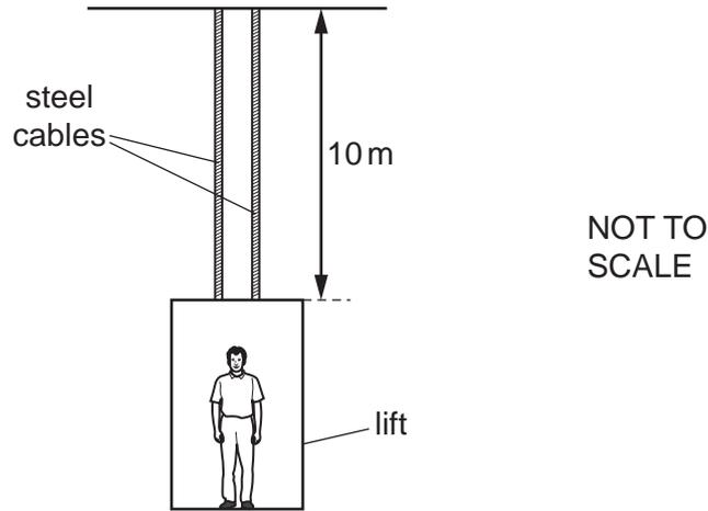
The cables extend by 1 mm when a man of mass 80 kg steps into the lift.
