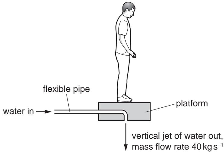
The resultant vertical force on the platform is zero. The combined mass of the man and platform is 96 kg. The mass of water that is discharged vertically downwards from the platform each second is 40 kg.
