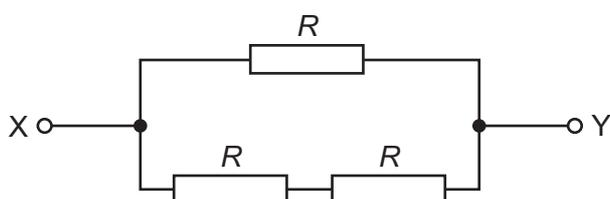
The total resistance between points X and Y is  $8.0\Omega$ .
