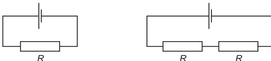
The cells in each circuit have the same electromotive force and zero internal resistance. The three resistors each have the same resistance  $R$ .
