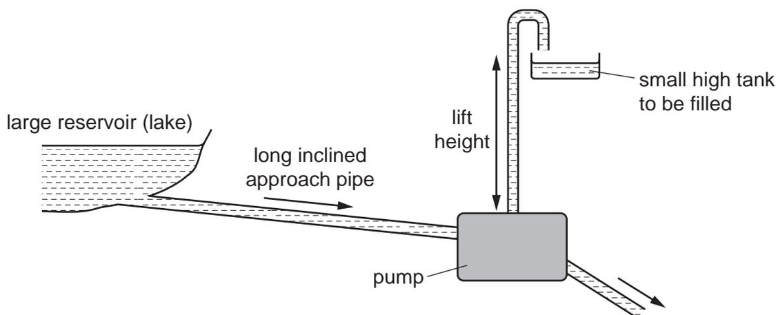
In one such pump the long approach pipe holds 500 kg of water. A valve shuts when the speed of this water reaches  $2.0 \text{ m s}^{-1}$  and the kinetic energy of this water is used to lift a small quantity of water by a height of 15 m.
