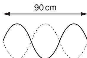
The frequency of the wave is 12 Hz.
