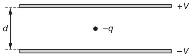
The separation of the plates is  $d$ . The droplet is observed to be stationary when the upper plate is at potential  $+V$  and the lower plate is at potential  $-V$ .
