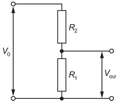
Which changes to  $R_1$  and  $R_2$  will increase the value of  $V_{\text{out}}$ ?
