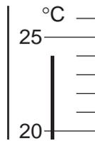
What is the correct reading on the thermometer and the uncertainty in this reading?
