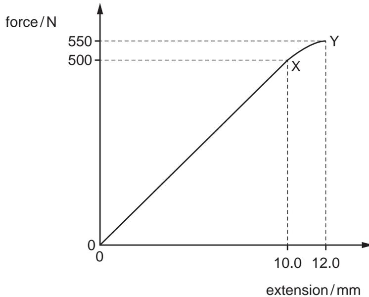
What is the total work done in stretching the sample from zero to 12.0 mm extension?
