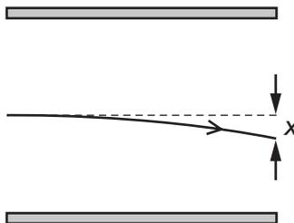
The vertical deflection  $x$  is measured at the right-hand edge of the plates.
