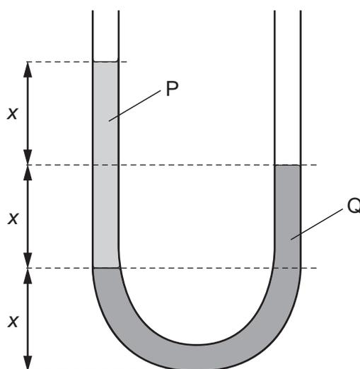
What is the ratio  $\frac{\text{density of P}}{\text{density of Q}}$ ?
