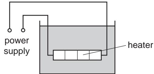
The heater has a resistance of  $3.0\Omega$ . The power supply has an e.m.f. of  $12\text{V}$  and an internal resistance of  $1.0\Omega$ .
