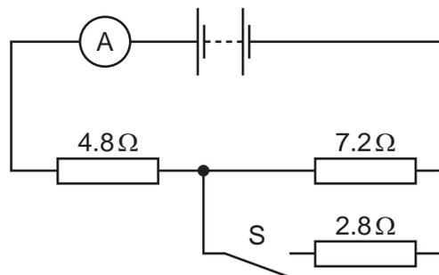
When S is open, the reading on the ammeter is 250 mA.
