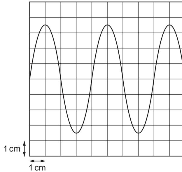
The oscilloscope time-base setting is  $0.5 \text{ ms cm}^{-1}$  and the Y-plate sensitivity is  $2 \text{ V cm}^{-1}$ .
