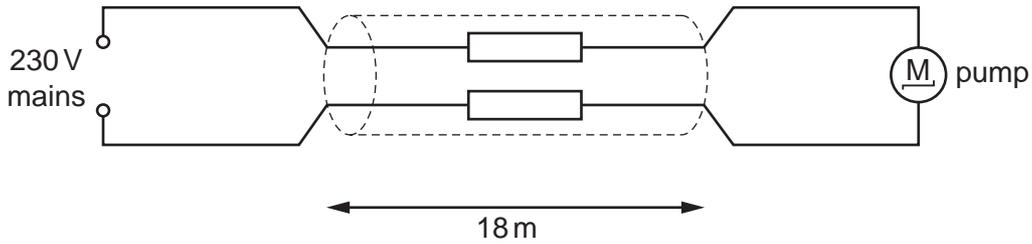
The performance of the pump is acceptable if the potential difference (p.d.) across it is at least 218 V. The current through it is then 0.83 A.
