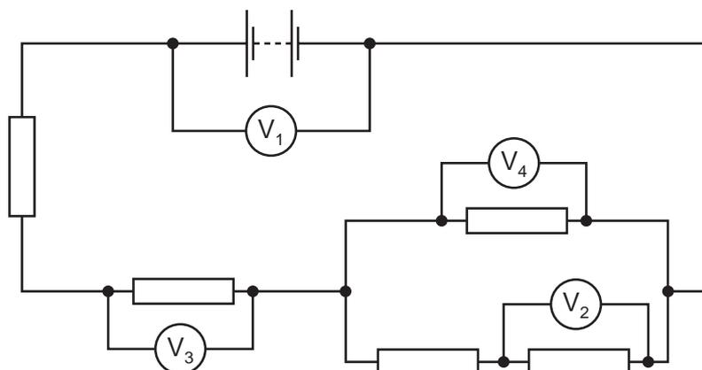
The reading on voltmeter  $V_1$  is  $8.0\text{V}$  and the reading on voltmeter  $V_2$  is  $1.0\text{V}$ .
