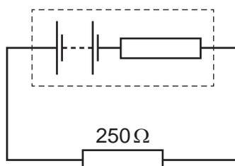
The current in the resistor is  $40\ \text{mA}$  for a time of  $60\ \text{s}$ . During this time  $6.0\ \text{J}$  of energy is lost in the internal resistance.
