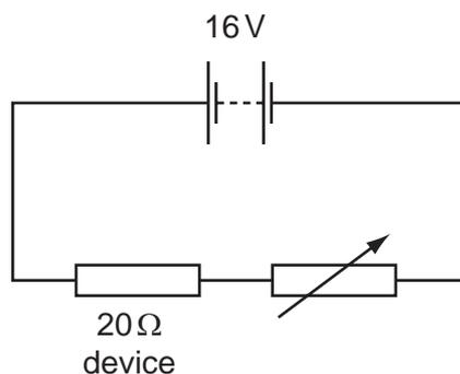
What is the resistance of the variable resistor when the power dissipated in the electrical device is  $4.0\ \text{W}$ ?
