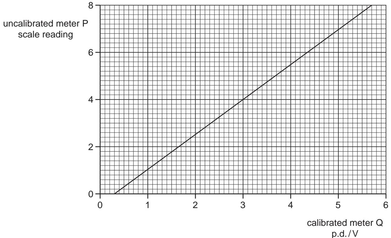
The graph shows that meter P has a zero error. This meter is now adjusted to remove this zero error. When the meter is recalibrated, the gradient of the calibration graph is found to be unchanged.
