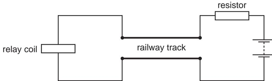
With no train present, there is a current in the relay coil which operates a switch to turn on a light. When a train occupies the section of track, most of the current flows through the wheels and axles of the train in preference to the relay coil. The switch in the relay turns off the light.
