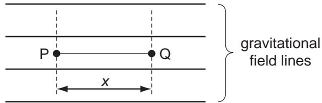
When the mass moves through a displacement  $x$ , from P to Q, it loses an amount of potential energy  $E$ .
