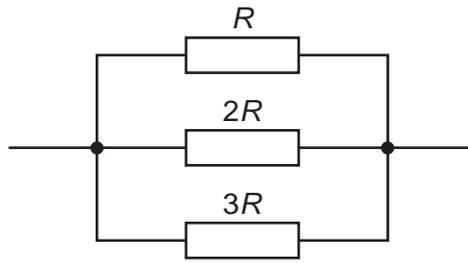
Using  $I$  to represent the current through the resistor of resistance  $R$ , which row represents the relationships between the currents through the resistors?
