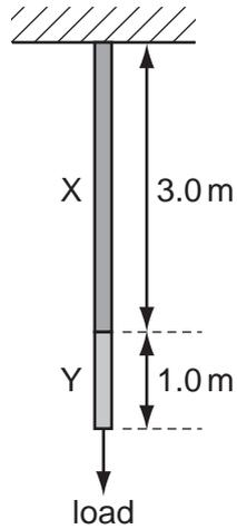
A load hung from the wire causes metal X to stretch by 1.5 mm and metal Y to stretch by 1.0 mm.
