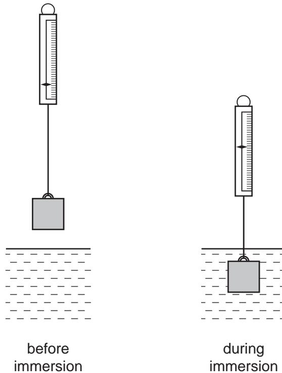
A reduction in the balance reading occurs as a consequence of the immersion.
