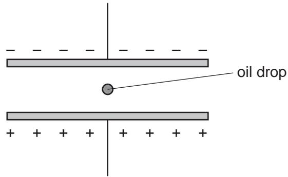
The potential difference across the plates is  $V$  and the separation is  $d$ .
