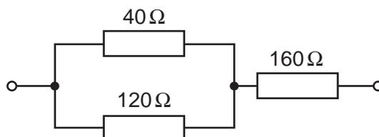
What is the total resistance of the combination of the three resistors?
