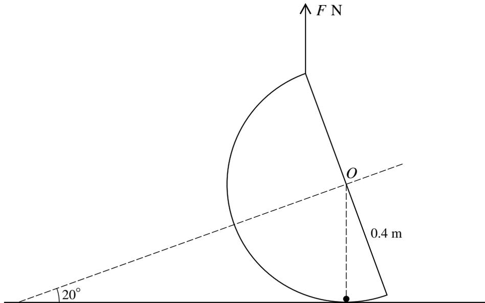
A smooth hemispherical shell, with centre  $O$ , weight  $12 \text{ N}$  and radius  $0.4 \text{ m}$ , rests on a horizontal plane. A particle of weight  $W \text{ N}$  lies at rest on the inner surface of the hemisphere vertically below  $O$ . A force of magnitude  $F \text{ N}$  acting vertically upwards is applied to the highest point of the hemisphere, which is in equilibrium with its axis of symmetry inclined at  $20^\circ$  to the horizontal (see diagram).
