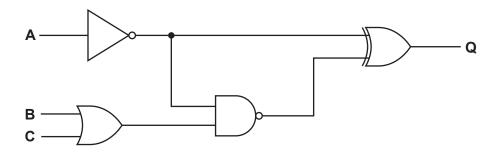
(a) Complete the truth table for the logic circuit.
